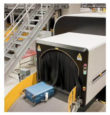
attention to the design of its solutions for the integration of the last generation baggage screening machines (Standard 3). The design of the layouts of baggage handling systems always keeps into account both the requirements for the security related "waiting times" and the needs for a fast flow of the "clean" bags, in order to achieve the highest possible throughput with the maximum-security level.
